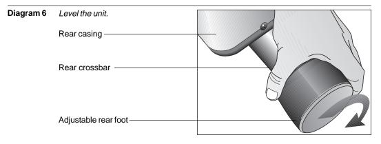
**Note**: You have completed the assembly of the EFX556. To level the unit and connect it to a power source, continue with the steps below.
